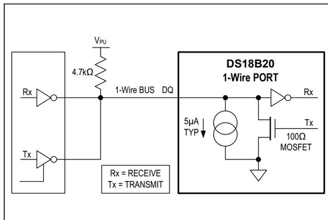
Figure 12. Hardware Configuration
