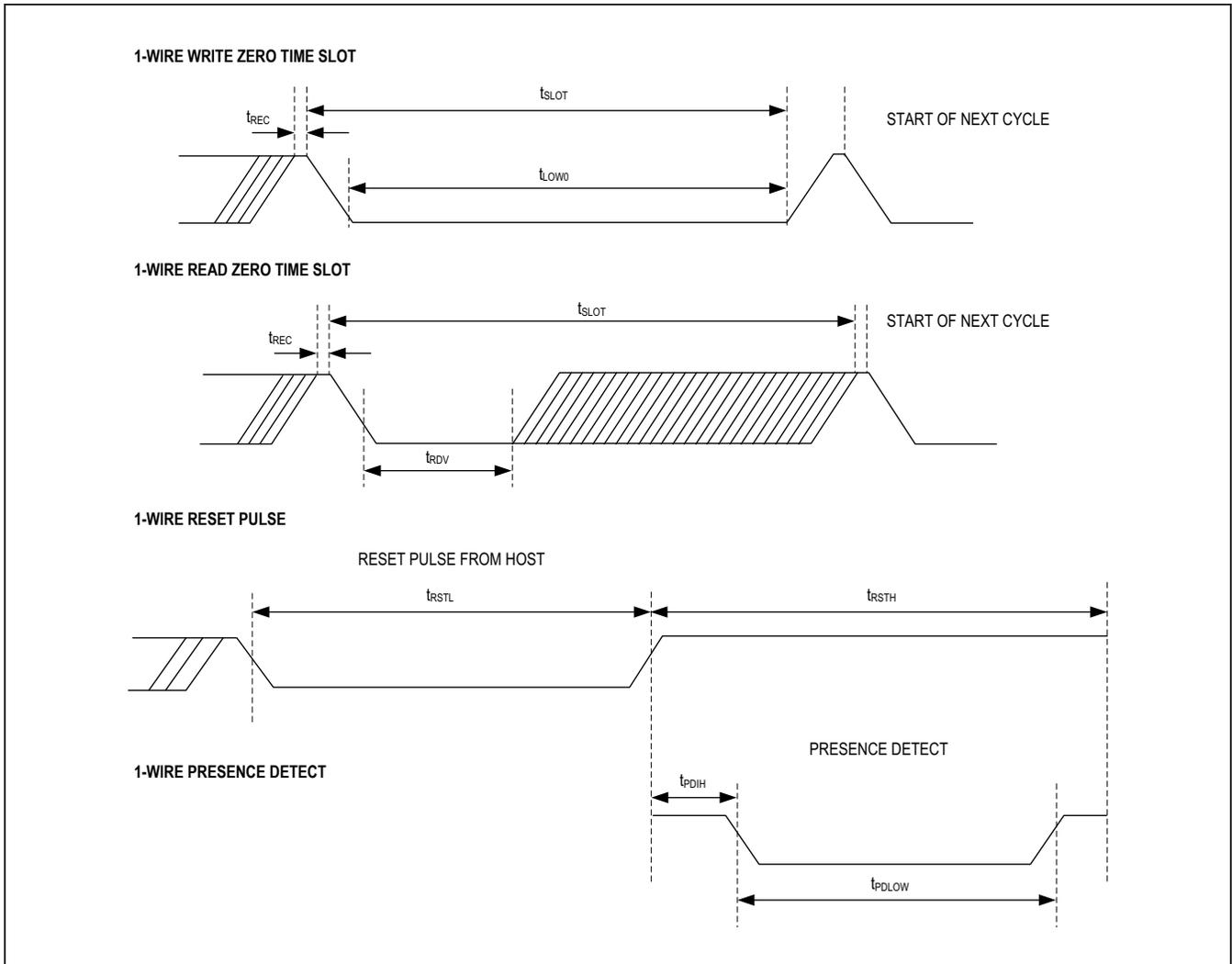
Figure 2. Timing Diagrams
