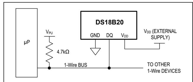
Figure 7. Powering the DS18B20 with an External Supply
